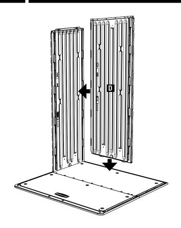
Using a screwdriver, punch out the screw holes on the top of Left Back (D) 4 places.
